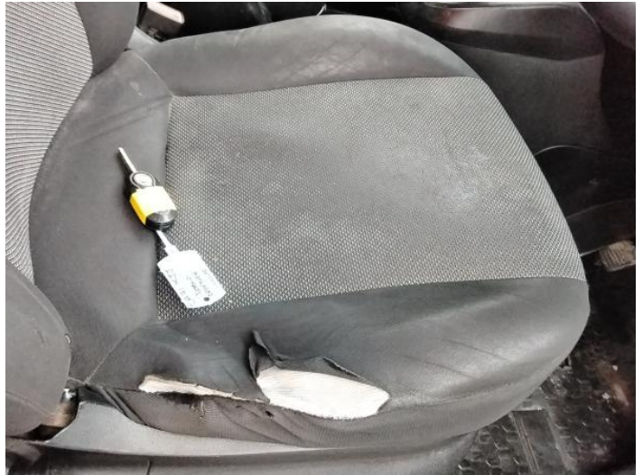
16: Seat Base Cover osf Torn Over 3mm
