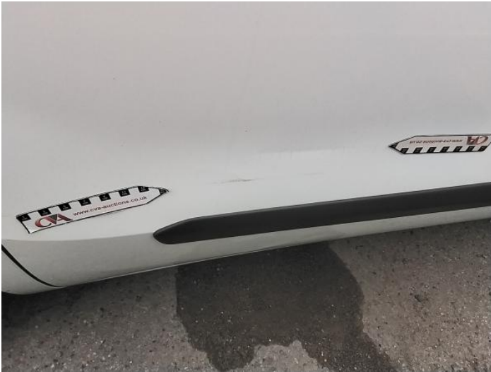
3: Door nsf Dented Over 30mm
