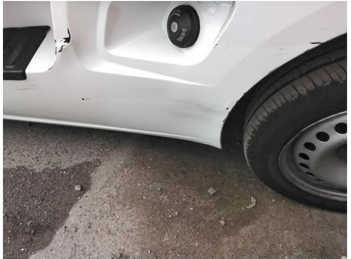
4: Qtr Panel nsr Dented Over 30% Of Panel
