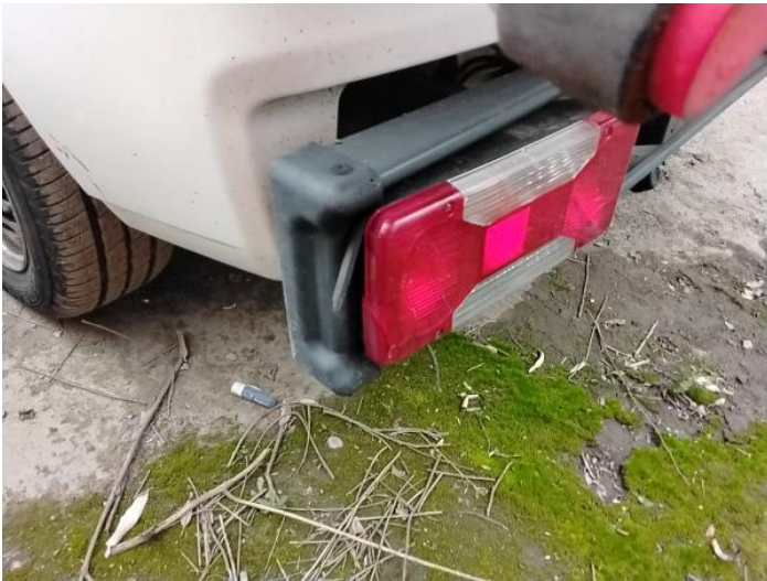
5: Lamp nsr Broken Replace
